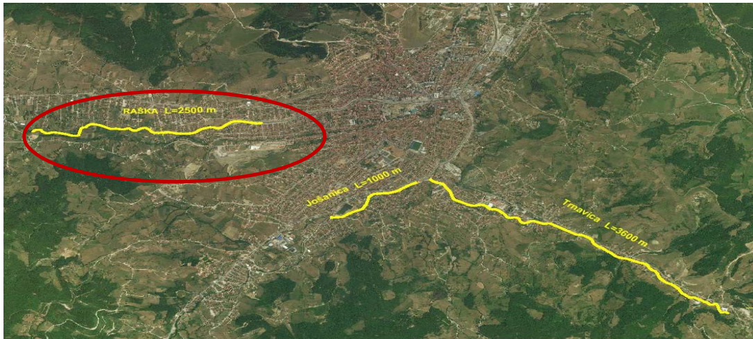
Figure 2 - Layout of Raška River Training works shown on contemporary satellite images
