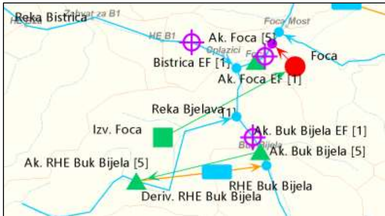
Figure 3-6: Representation of the pumped-storage HPP Buk Bijela in the Drina WRM model.
