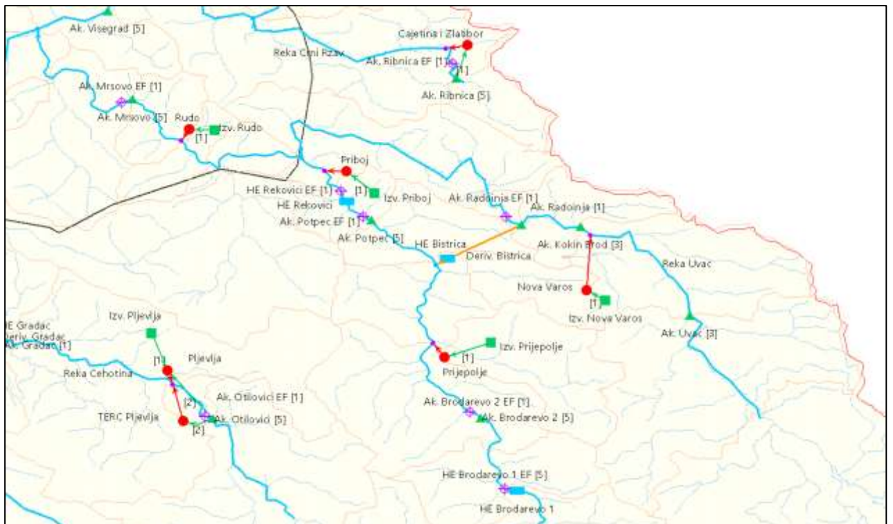
Figure 3-4: Detail of the schematic of the Drina River Basin water resources system in WEAP (Uvac River).
