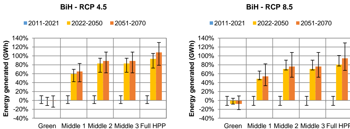
Figure K-8: Combined climate change and development options effects: change in average annual hydropower generation in BiH (excluding joint HPPs with Serbia) relative to 1961-1990; ensemble medians with ranges of results from different climate models for RCP 4.5 (left) and RCP 8.5 (right) climate scenarios.
